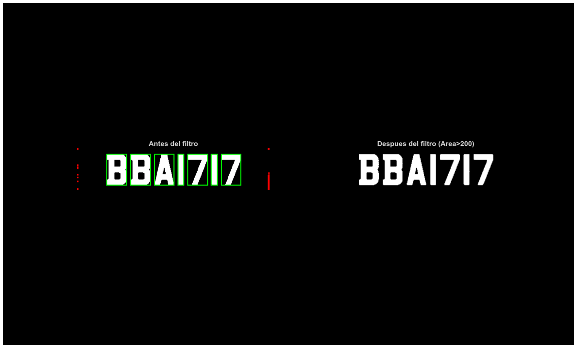
Figure 8: Components of the plate region before and after the filter. In green, the seven valid characters. In red, residual noise dots and a piece of the frame line, discarded by the Area > 200 filter.
